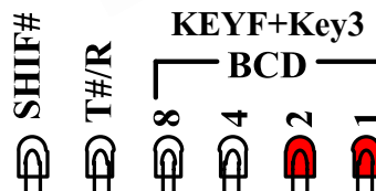
Figure 3.3 shows example of status at PINs of Connector 8PIN when pressing Key F together with another Key (Key F+Key3).
